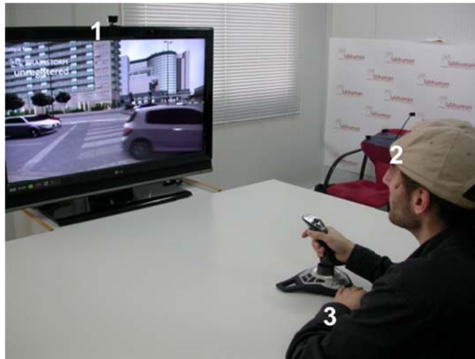
Figure 2. Hardware setting of the VR system. 1) TrackIR™ camera; 2) Clip of reflective marks; 3) Joystick.
