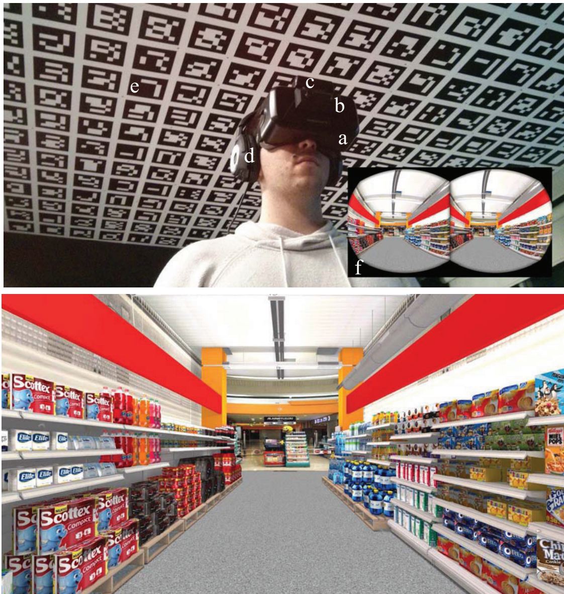
Fig. 7. User interacting with the proposed virtual reality system. Top: Experimental setting. a) Oculus DK2; b) Ovrvision; c) Playstation Eye camera; d) Kinivo BTH220; e) pattern of fiducial markers; f) virtual environment that is being displayed. Bottom: Snapshot of the virtual environment (grocery store) where user is immersed.
