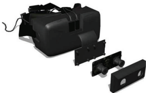
Fig. 5. Attachment of the Ovrvision to the Oculus DK2.
